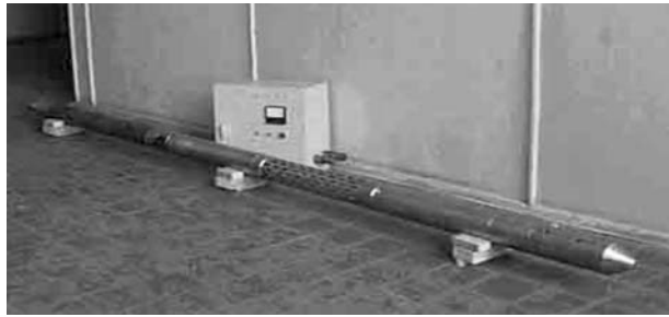
Fig. 4. Device for US treatment of water-supply wells with submersible unit 108 mm in diameter.
