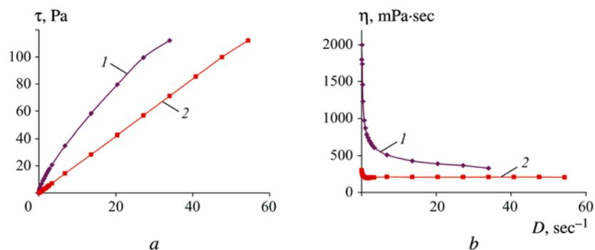
Fig. 1. Dependence of shear stress  $\tau$  (a) and viscosity  $\eta$  (b) on shear rate  $D$ : 1) initial crude; 2) sample 10.
