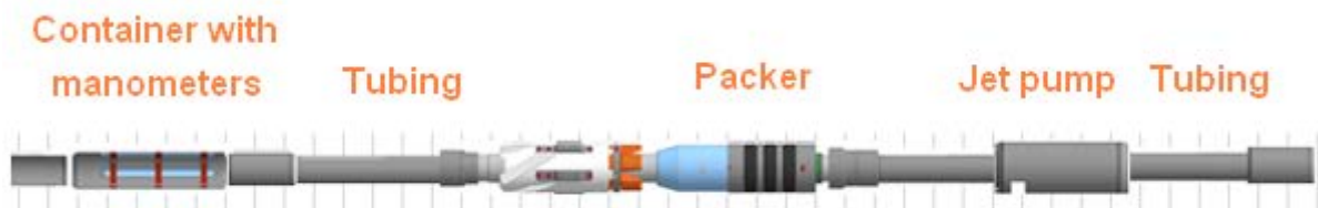
Fig. 7 Configuration of downhole equipment during treatment
